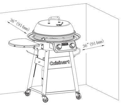
\Lambda This griddle is intended for use outdoors and must not be used in a building, garage or any other enclosed or covered area.
