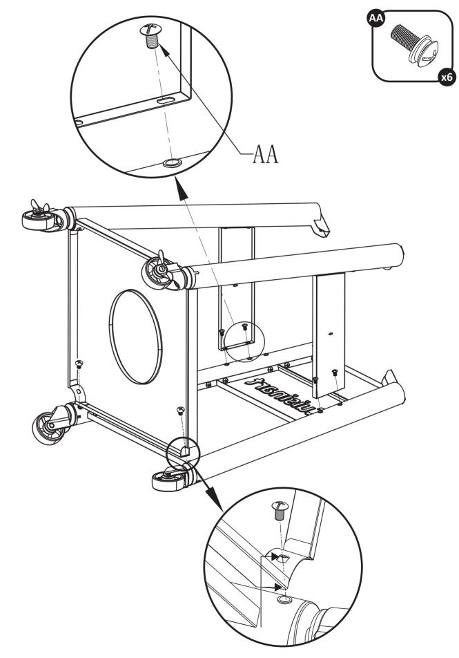
5. Put the griddle's body onto the stand and align it with screw holes on each leg. Secure each leg with M6 screws (AA) and washers (FF).
